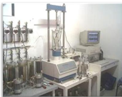
STRENGTH TEST : CONSOLIDATED UNDRAINED TRIAXIAL TEST (CIU)
