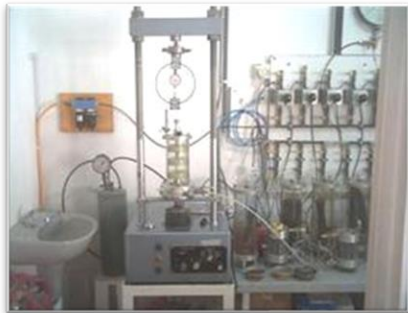
STRENGTH TEST : UNCONFINED COMPRESSION TEST (UCS) & UNCONSOLIDATED UNDRAINED TRIAXIAL TEST (UU)
